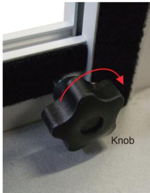
Turn knob clockwise to tighten lock.
